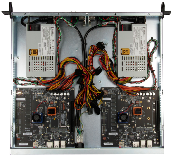
Figure 1: The Monte Cimone Server Blade hosts two SiFive Freedom U740 SoCs and has a form factor of 4.44 cm (1 Rack-Unit) in height, 42.50 cm in width, and 40 cm in depth. Each RISC-V board has dimensions of 170 mm by 170 mm. Image from [5].
